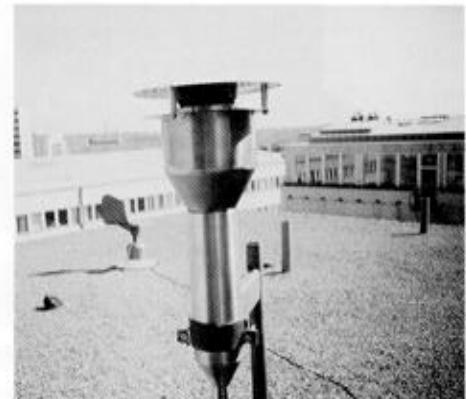
Fig. 2.2 University of Minnesota type inlet of a static size-selective bioaerosol sampler.
